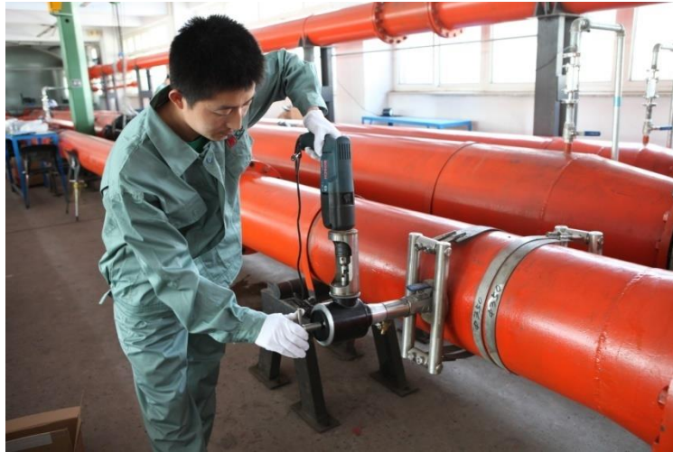
Picture 4-17 Schematic Diagram Showing the Drilling Operation
