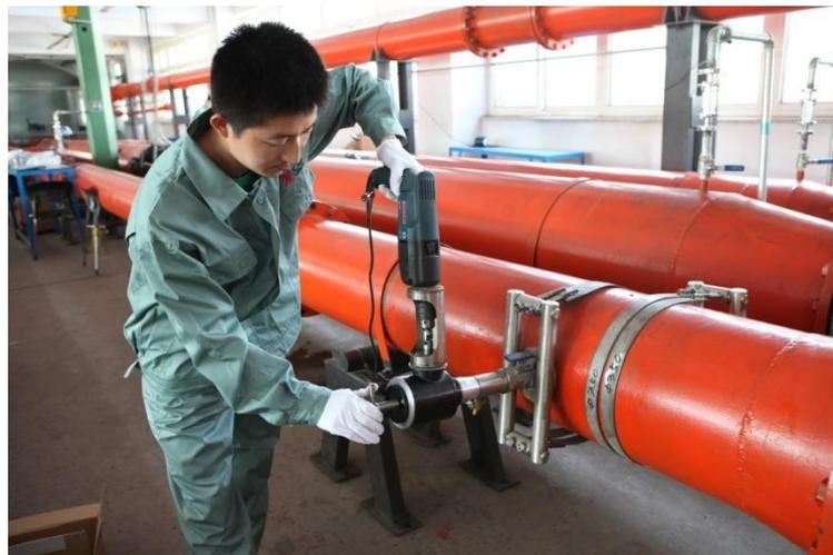
Picture 5-12 Schematic Diagram of Drilling Operation
