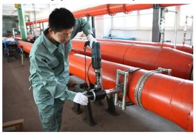
Picture 5-14 Schematic Diagram of Drilling Operation
